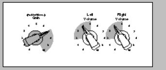
For vintage blues tones, keep the Gain in Normal mode (pushed in), but crank it up to 7 or so to push the power amps harder. You'll notice that the amount of "sag" (power amp compression) increases as you turn the Volume controls beyond 5. When set up this way, the Signature 284 is most responsive to nuances of touch and style — the tone is totally authentic, the voice is yours alone.
